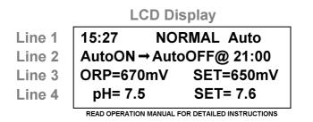
Line 1 shows the current time and the mode of operation. In the example above, line 1, tells you that the time is 3:27pm and the PL Twin System is operating in "Normal Automatic mode" Note that the PL Twin System displays the time using a 24 hour clock.
