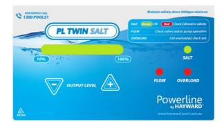
The PL Twin Salt Unit uses a simple LED Bar Meter and Alarm LEDs to provide the user with information. There are 3 buttons to make adjustments to the system: ON/OFF, +INCREASE & -DECREASE.
