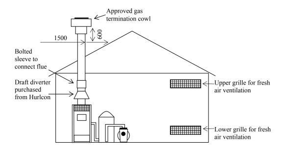
An indoor draught diverter must be purchased from Hurlcon and fitted to unit in accordance with Hurlcon's Instructions and Installation Codes before the heater can be enclosed.
