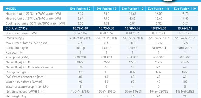
\*Heating: 27°C air / water 26°C / humid 80% \* The data above is based on the EVO heat pump only, it does not include auxiliary devices. Product specification information provided above is correct at the date of printing, this data may change without notice. Please speak with an EvoHeat Specialist for the most current product specifications.
